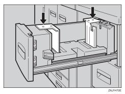
**4** Fasten the side fence with the screw.
